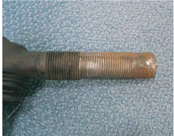
Thread Damage - Loose Clamp Assembly
