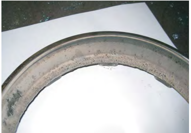
Bearing Cup - Water Contamination
