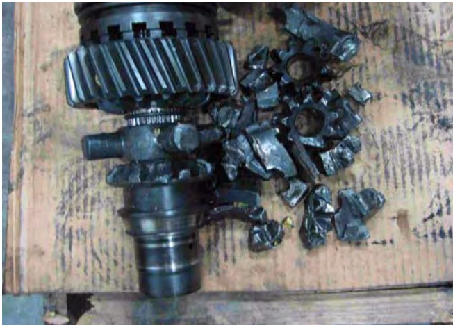
Input Shaft Assembly - Catastrophic
