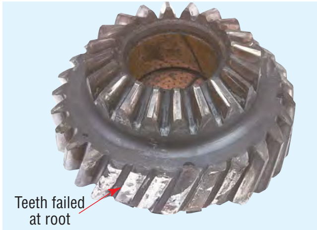
Input Shaft - Torsional Shock Failure
