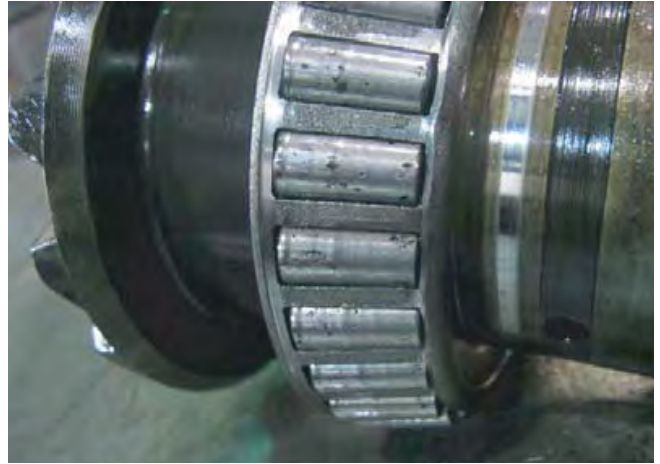
Bearing Cone - Spalling - Water Contamination
