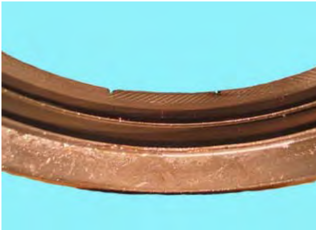
Damaged Seal Lip
