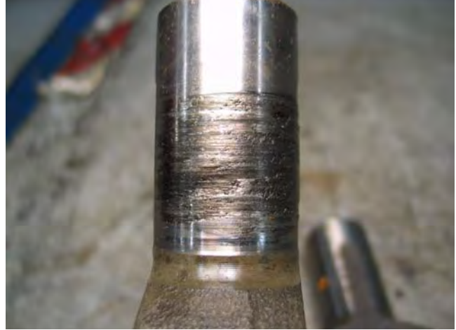
Thrust Washer to Input Shaft - Galling
