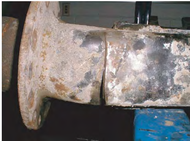
Housing Arm Fatigue
