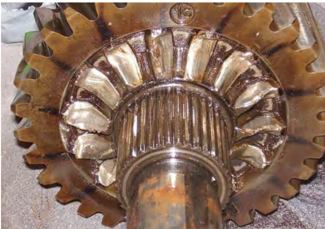
Helical Side Gear Wear - Water Contamination
