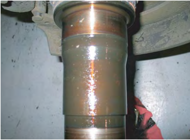
Housing Arm Fatigue
