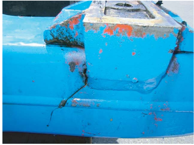
Hanger Bracket Fatigue
