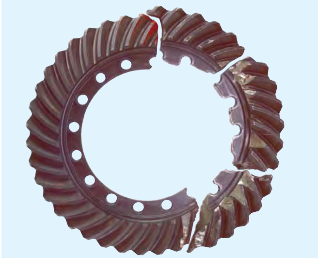
Drive Pinion - Torsional Shock Failure
