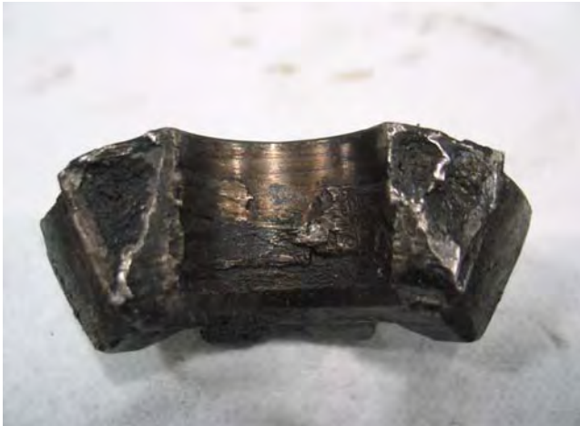
Input Shaft Assembly - Catastrophic
