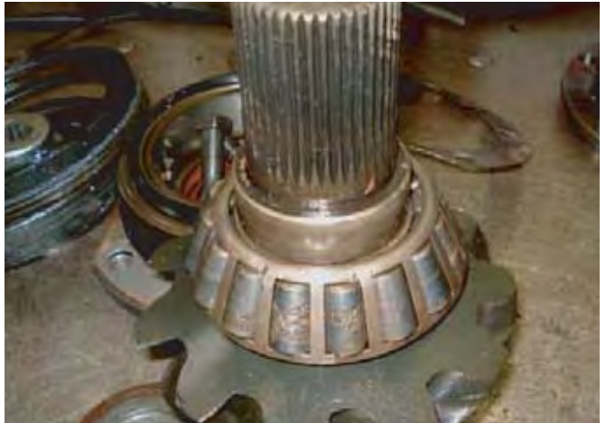
Bearing Cup - Water Contamination
