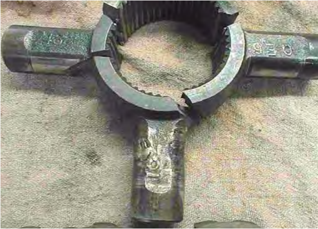
IAD Spider Arm - Bore Galling
